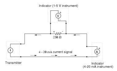
possible for a properly functioning system then is only 16 mA (20 mA – 4 mA). This 16 mA range is known as the "live signal." The actual reading being recorded in mA is called the "process variable." The PV indicates a percentage of a particular measurement being monitored. The table below shows the relationship between various PVs and their corresponding percentages.
